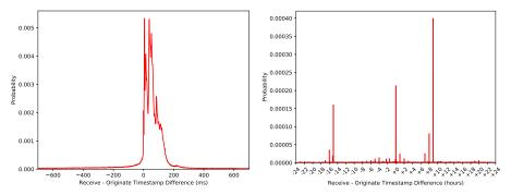
Fig. 4. Empirical recv\_ts- orig\_ts PMF Fig. 5. Response error; note hourly peaks
